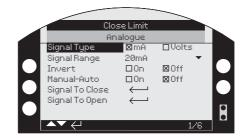
When analogue control is selected independent deadband and hysteresis adjustments are provided in the menu to optimise the control to suit the process conditions. The position against demand profile can also be tailored to suit the specific valve flow characteristics such as linear or equal percentage profile by utilising the Rotork Insight2 software.
