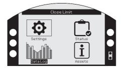
The data can be viewed locally on the dot matrix display and can display pressure and position graphs through to statistical operational data. All data held is secure and can be down loaded using the Rotork *Bluetooth*<sup>®</sup> setting tool for viewing on a PC with Rotork Insight2 software.
