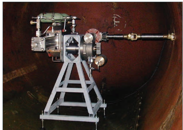
Hydrostatic qualification for subsea gearbox.
