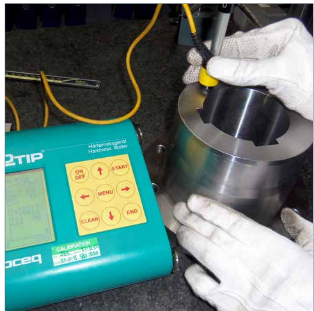
Hardness check of drive sleeve with Equotip hardness tester.
