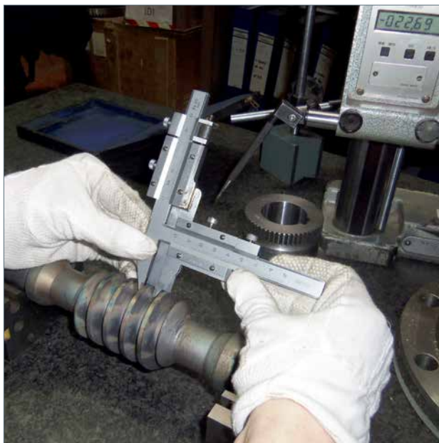
Gear teeth dimension check with vernier gear tooth.
