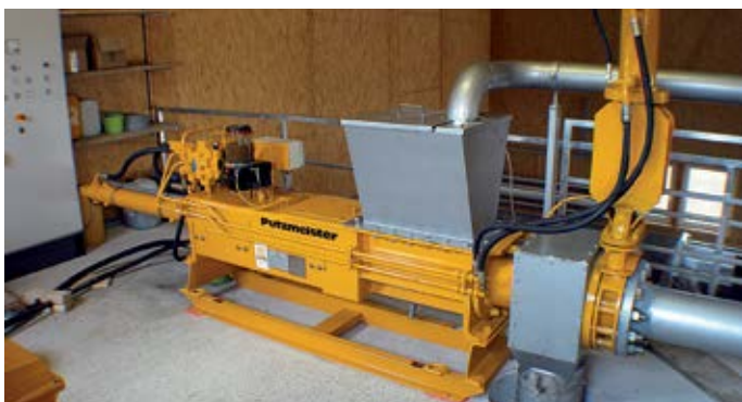
EKO 1060 PP at the biomethanisation plant in Kössen (Austria) for the transportation and de-wrapping of expired food
