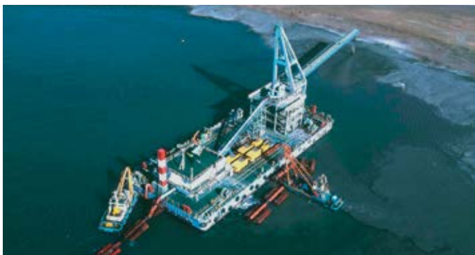
Three huge piston pumps KOS 25100 und 25200 are pumping silt out of the sea for arising an artifical island in front of the japanese coast line
