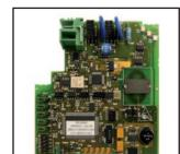
The FlexLine series is now available as a HART compatible device. This allows the FlexLine to be connected to any operational interface or other device that supports HART. All level information, parameters and diagnostics can be transferred to the operator HMI via this interface stack. The HART information can also be routed via the OneWireless infrastructure. Due to the modular architecture of the FlexLine, multiple HART interfaces can be integrated into one gauge.
