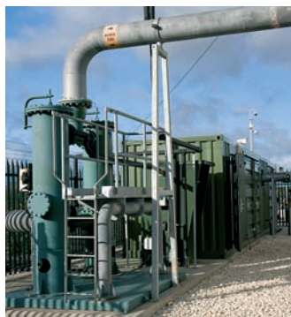
Compact mine gas compressor station in a container.
