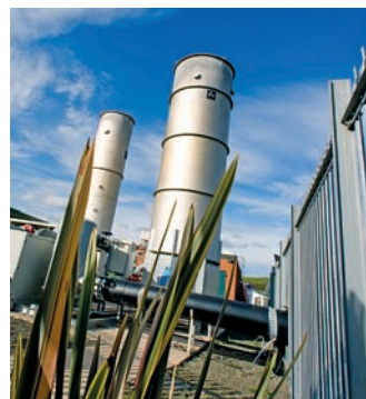
Modular degassing plant for landfill sites, with high-temperature combustion.
